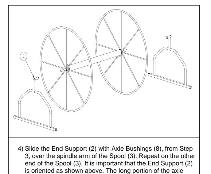
housing should face toward the Wheel Hubs (4).
