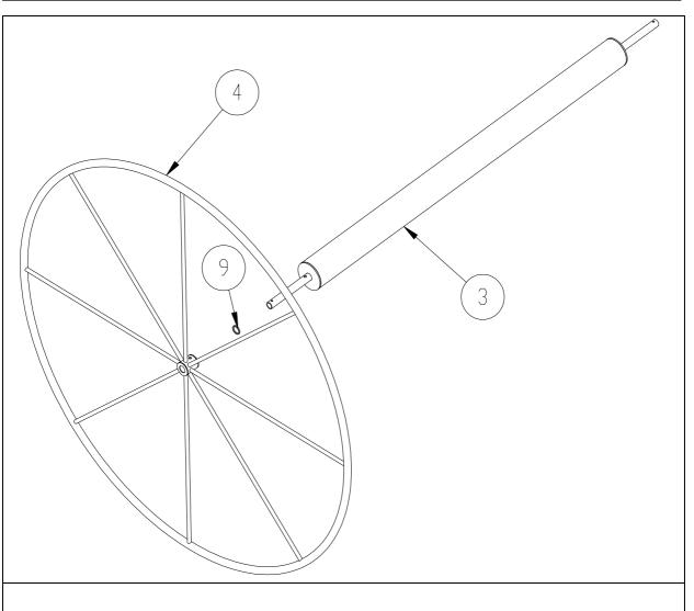
The lid of the cardboard box that the unit was shipped in works as an ideal surface to assemble the lane line reel. First, slide the O-Ring (9) over the spindle arm of the Spool (3), and then slide the Wheel Hub (4) over same side of the Spool (3). Repeat this on the other end of the spool. The finished assembly should not be placed on the ground because this can damage the powder coating.
