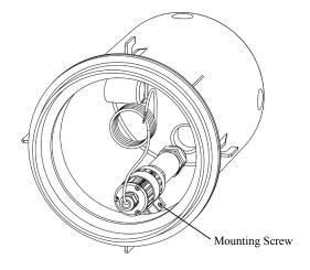
Insert the Fiber Ferrule into the LED Driver until you cannot push the ferrule any farther. **HAND** tighten the LED Strain Relief. Remount the LED driver into the mounting bracket in the reverse order as discussed in the previous step.
