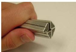
While holding the ferrules together, insert into the strain relief opening as illustrated.
