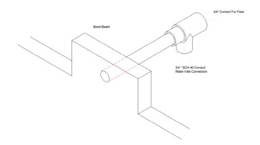
**Note:** DO NOT INSTALL THE AQUA ACCENT DELUX TIP MORE THAN 4" THROUGH THE GUNITE SURFACE AREA. THE INTERIOR OPTIC ROD IS 4 ¾" DOWN FROM THE TIP'S TOP AND WILL BE DAMAGED IF TRIMMED FOR FLUSH INSTALLATIONS BELOW THIS LEVEL.
