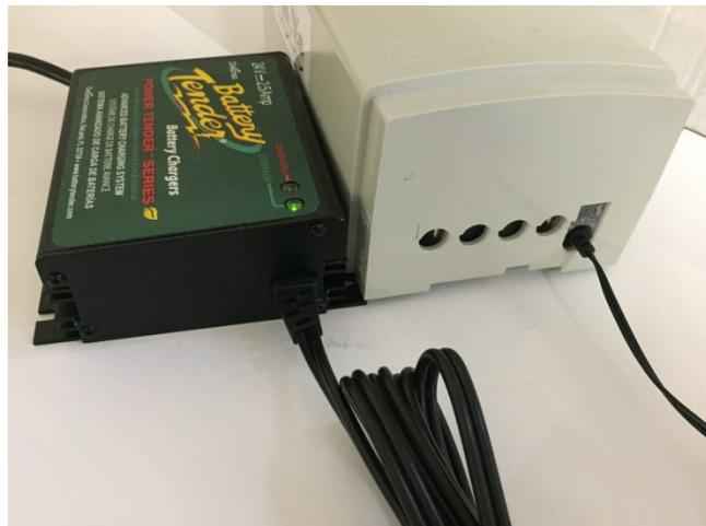
continues to flash, either the battery voltage is too low (battery pack needs to be replaced), or the battery charger is not properly connected to the battery.
