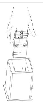
(5) If the product is not being reinserted into the anchor, once the wedge is in place tighten it using the Allen wrench. Insert the wrench into the anchor bolt and turn clockwise one turn to gently tighten the wedge into place. NOTE: Do not over-tighten.
