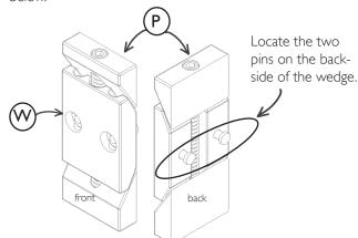
3 The pins align into the two slots on the back inside wall of the anchor.
