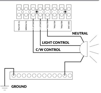
If this product is used to connect underwater lights directly, refer to 1999 NEC 680-21(b), 2002 NEC 680-24(b) or CEC 68-060, 062 and 066 for details.
