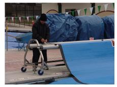
6. Prevent abrasion by rolling cover(s) evenly onto the reel, avoiding 'telescopic' effect. Secure it by attaching cordage around the rolled-up covers.
