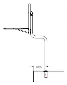
5. The Single Post Basketball units are to be anchored to the deck using a 6-inch deep AS-100D anchor socket or the AS-100P plastic anchor socket, with tightening bolt. Install the anchor in the pool deck 12 inches back from the pool's edge as shown in **FIGURE 5**. Properly bond the anchor socket using the attached bonding screw and the appropriate bonding wire per local codes. Allow concrete to cure before installing Single Post Basketball Unit.
