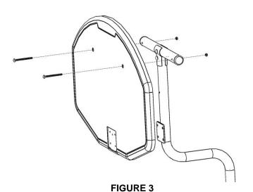
with the holes in the horizontal support tube as shown in **FIGURE 3**. Insert the 5/16" x 4" cairrage bolts into each hole in the backboard and through the horizontal support tube. Thread a hex nut onto the end of the carriage bolt that passes through the backside of the horizontal support tube. Do not tighten the hex nuts all the way down at this point.
